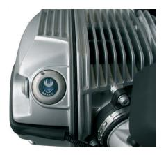
There is a drilling in the side of the plug in which you can put a size 3 Allen key or a Torx key T10 (usually found in the your BMW toolkit) in order to fit and remove it. See tools
