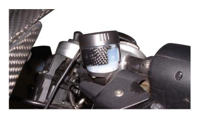
Cover kit for reservoirs of brake and clutch fluid with carbon surface. The carbon fibre parts are precisely shaped and are to be fitted by glue.
