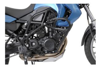
Our crashbars are made of high-quality steel and are specially designed for your F650GS, F700GS and F800GS 2008 model or newer. The crashbars are designed to be very robust and allow an equal distribution of the forces so that you and your bike are protected in the best possible way. Crashbars offer a very good protection but they can reduce the cornering angle.
