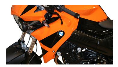
This Radiator Cover is either made of glass fibre reinforced plastic (GRP) or high quality carbon fibre. It covers the radiator and its tubes. The GRP cover is black primed.
