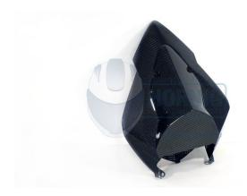
This Racing Seat Unit is made of high quality carbon fibre. The article number SIO.062.S1RAB.K (as well as SIO.085.S1RAB.K) has a very high quality powder coating. The Seat Unit is specially made for the race track and has no street homologation.
