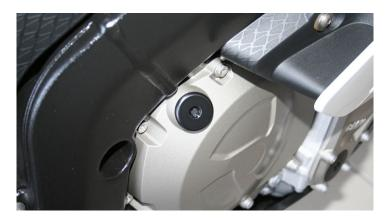
This Oil Filler Plug is made of high quality aluminum and available in black anodized or silver anodized. You can open this Oil Filler Plug with a Torx T45.
