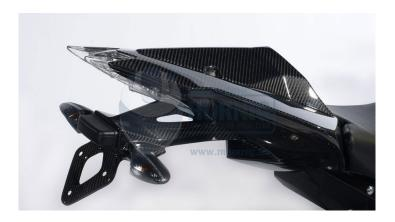
These two parts for the tail of the BMW S1000RR are made of high quality carbon fibre and covered with UV resistant clear lacquer. The article numbers SIO.015.S100S.K and RHA.014.S100S.K have an ABE/street homologation.
