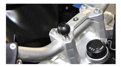
You screw the GPS ball into the upper triple clamp. The screw is 55/60/65mm long with a M8 thread.
