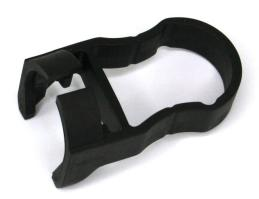
The spark plug connector of the new generation bikes makes it easy and secure to remove the spark plug connector. The connector is actually the coil as well. This tool makes it easy to remove the spark plug connector / high tension coil. Attempting to remove the connector without the proper tool will not only be difficult, it may cause irreparable damage to the connector.
