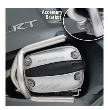
These stainless steel engine guards will, unlike powder-coated steel guards, never rust. They are carefully designed to allow clearance for oil changes or valve cover access, so they never need to be removed. Guards attach to the engine mounts, not the engine covers, to protect the engine heads and not destroy them. Integrated top brackets on each guard allow the rider to mount accessory lights, video cameras, or whatever they can imagine!
