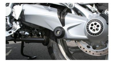
This crash-protector for the cardan is made of cnc lathed plastic. This crash protector provide additional protection for your motorcycle. You install the crash protector or pad on your cardan with a stainless steel screw and an expansion holder.
