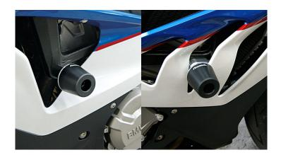
These crash protectors are the latest design-version of the EQ704 crash protectors. They offer the best possible protection if a crash was not avoidable. The brand new compound plastic can absorb forces of a crash without braking. But these crash protectors are not only very usable but also good looking. The crash protectors are for left and right side and you can mount them quite fast and easy. They come with a special holder so no drilling or cutting the fairing is necessary.
