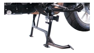
This main stand is characterized by its accuracy of fit and its stability. It is very instrumental in any little work you have to do on your bike just like changing the brake pads and so on...
