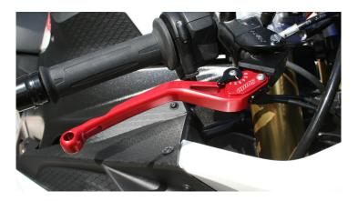
Synto is the name of the 6x adjustable CNC high-precision brake and clutch made of aluminium. Combines elegance and functionality. Handling pure!
