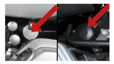
These covers for the open holes of the engine mounting are made of aluminium and available in silver anodized. These 4 covers will be installed in front of and behind the cylinder on the left and right side. Shipping contains a set (4 pieces).
