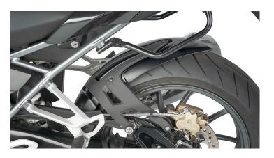
This solid rear hugger is made of ABS resin plastics and provides perfect protection for your suspension, your exhaust, your header and for the whole rear part of your bike. Not to forget your pillion rider! Also referred to as rear hugger, rear fender, rear splash guard, mud guard, mud protection Everything you need to install it is included. You can download the install instruction here. With ABE (European homologation).
