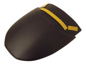
The rear section of the front fender is not long enough to effectively keep road debris off the exhaust and front of the engine. The fender extender solves this problem effectively and elegantly.
