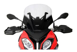
The touring shield has the same shape as the original windshield, but with an additional raised wind deflector about 5-7 cm high at the top, covering the entire width. This deflects the wind over the rider and allows a relaxed ride, particularly on longer trips.
