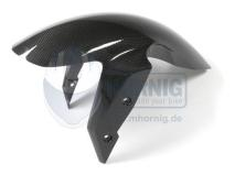
This front mudguard is an optical improvement for your BMW F800R (2015-). Made of high-quality carbon fibre which is usually used in motorsports. With EG/ABE homologation.
