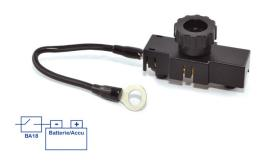
BA18 is a fully insulated battery master switch for bikes, scooters and quads. In long standing intervals it prevents the battery discharge through permanent power consumption such as board computer, watch, USB sockets, ...
