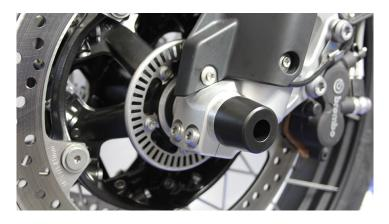
These crash protectors for forks are made of cnc lathed plastic (POM). The mounting is made of cnc milled and anodized aluminum. These crash protectors provide additional protection for your fork. Shipment includes the crash protectors (left and right) and the mounting. BMW RnineT (2016-2020) BMW RnineT Scrambler ( -2020) BMW RnineT Pure ( -2020) BMW RnineT Racer BMW RnineT Urban G/S ( -2020) BMW RnineT /5
