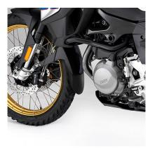
The rear section of the front fender is not long enough to effectively keep road debris off the exhaust and front of the engine. The fender extender solves this problem effectively and elegantly.
