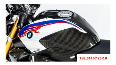
The carbon fiber tank cover for the BMW R1250R replaces the original piece using the original mounting points.
