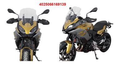
The touring shield is 4cm higher than the original windscreen. This windshield deflects the wind over the rider and allows a relaxed ride, particularly on longer trips.
