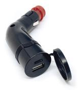
Our USB adapter for the motorcycle socket (USB10) adapts different 12/24V sockets to the USB standard of 5V to two USB sockets (USB-A and USB-C with max. 3,6A each). Usual USB adapters only fit for big cigarette lighter sockets. This USB adapter fits for both the big cigarette lighter socket and the smaller motorcycle socket like BMW uses it (DIN socket, article number 90025).
