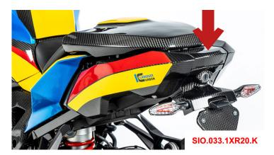
This rear fairing made of extremely resistant carbon fiber upgrades the look of your BMW S1000XR (2020-) & M1000XR a lot and, thanks to its light material, saves weight. The upper rear fairing is attached directly above the license plate holder and rounds off the motorcycle in an elegant way.
