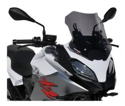
This windshield is made of sturdy acrylic (PMMA) and its height (35cm) offers optimal wind and weather protection. This enables relaxed and comfortable driving, even on long tours. The windscreen is tinted dark (transparent) and is attached to the original mounting points. It was made in Europe and has a street homologation.
