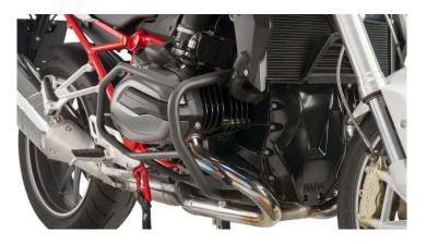
Our crash bars are made of high-quality steel and are sepcial designed for your BMW R1200R LC & R1200RS. The crash bars are designed to be very robust and allow an equal distribution of the forces so that you and your bike are protected in the best possible way. Crash bars offer a very good protection but they can reduce the cornering angle.
