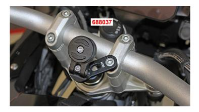
The SP Connect Bar Clamp Mount Pro is the perfect way to attach your smartphone to the motorcycle in a matter of seconds, flexibly and intuitively. The Bar Clamp Mount Pro can be mounted on the handlebar clamp and offers a pivoting and rotating head in order to be able to position the smartphone optimally. The smartphone can be fixed in both portrait and landscape format.
