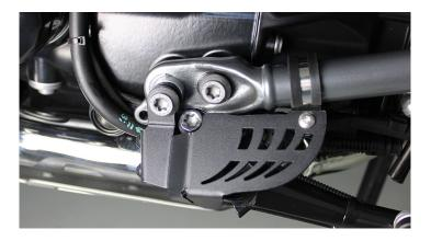
Aluminum protective cover for the safety switch on the side stand.
