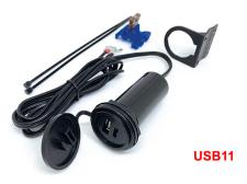
This USB twin on-board socket (2x maximum 3.6A) is equipped with a USB-A and a USB-C socket and is therefore ideal for charging modern smartphones. The socket converts the input voltage from 12/24V to the USB standard of 5V and has a 1.5 m long connecting cable. The socket can be flexibly mounted on the handlebar or tubular linkage using cable ties.
