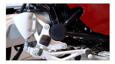
This cover is the perfect replacement for the original plastic cap. Made of aluminium. BMW R1200R 2005-2014
